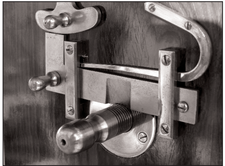
Figure 8. The mechanism to set the barrel in eight different positions
